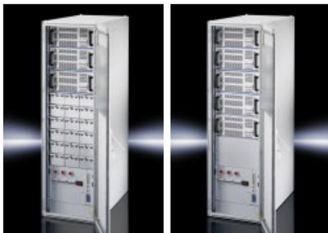
Rittal PMC 200 ensures optimum availability for critical applications by combining modularity (flexible, unlimited scalability and redundancy, whereby up to 20 modules may be switched in parallel) with decentralised parallel architecture or DPA (redundant protection without a "single point of failure"). The UPS modules are transformerless, genuine online, double-conversion UPSs with static bypass and classification code VFI-SS-111.
